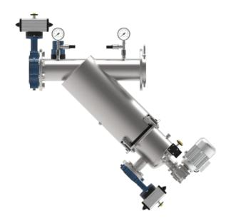
WONDERJET is a self-cleaning mesh filter, suitable to treat fluids loaded with a medium-high amount of suspended solids, even colloidal. WONDERJET, thanks to powerful pressurised water jets, efficiently cleans the filtering element in a short time and with reduced water consumption.
