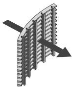
**OW** – slot parallel to the axis, flow from inside to outside (FITO)
