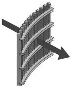
**RW** – slot parallel to the axis, flow from inside to outside (FITO)
