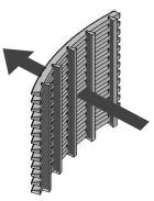
**RZ** – slot parallel to the axis, flow from outside to inside (FOTI)
